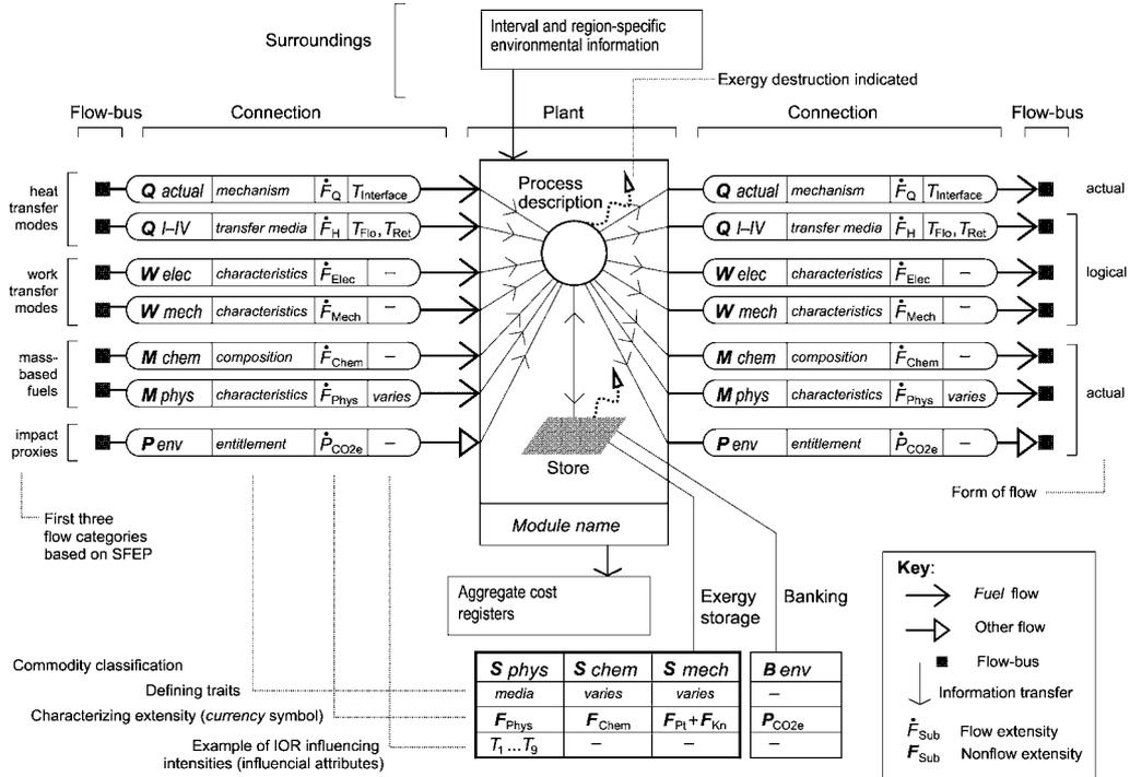
Figure 4. A generalized plant/connection/flow-bus. The classification of *fuel* connections arises directly from the SFEP concept. Multiple flows of each type are possible although indexing will be needed. Note the presence of non-engineering commodity types – for instance, environmental impact entitlements.
