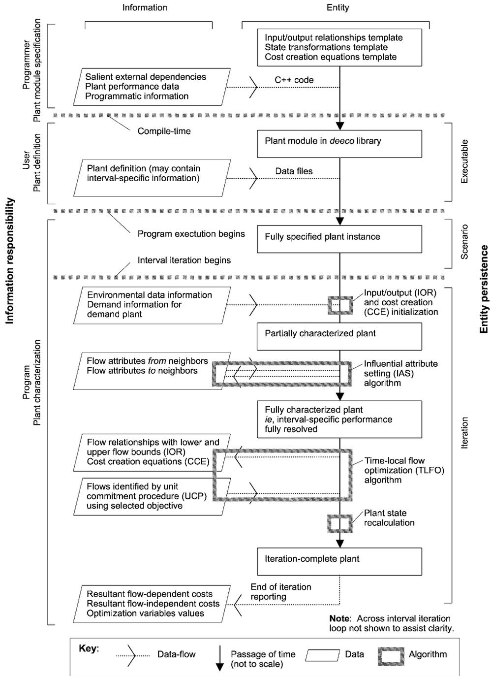
Figure 5. The lifecycle of a plant as per the current release of *deeco* – from the perspective of that plant. This diagram also indicates the staging of key procedures during any given time-interval and thereby depicts the temporal relationships between many of the ideas presented in section 8. *Source:* [43, figure 8.6].
