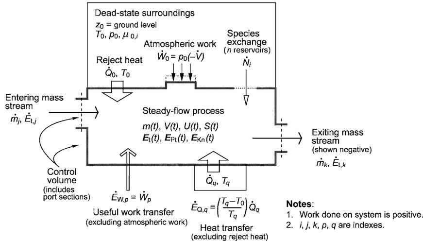
Figure 3. A generalized steady-flow exergetic process (SFEP) whose extension as a dynamical entity would be interpreted as a sequence of *non-stationary* SFEP. This entity is the building block from which plants are formed and from which *fuel*-based commodities are categorized. Some notation is given in footnote 12, otherwise the symbols have their usual meanings. *Source*: adapted from [4, chapter 5].
